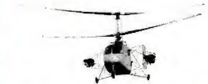
Wingless convertiplane flown two years ago by Gyrodyne was a coaxial helicopter fitted with a pair of outrigger engines
